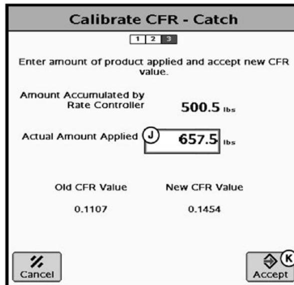
Depending on the type of product being dispensed and the accuracy of the weighing system, the CFR test may need to be carried out 2-3 times. The more CFR tests, the more accurate the CFR value.
