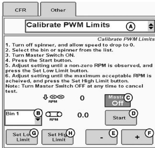
Follow the on screen instructions to set the low and high limits. Before starting the calibration procedure ensure that hydraulic feed belt drive is connected to the tractor remotes and that **25 L/Min** of oil flow is allocated to the feedbelt circuit. Oil flow should be turned on and the tractor engine running at normal operating speed.
