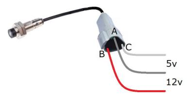
Test 2: Metal in front of tip, LED is on, multimeter on A+B shows 12v, multimeter on A+C shows 0v to 1v
